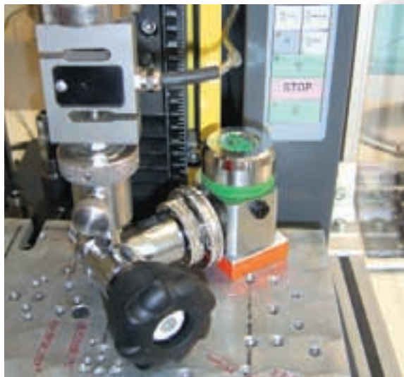
The shear and bending strain resistance is tested by a special machine with forces up to 2,000 N
